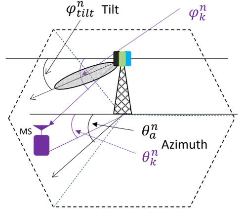
Figure 1. Illustration of antenna tilt and azimuth angle
