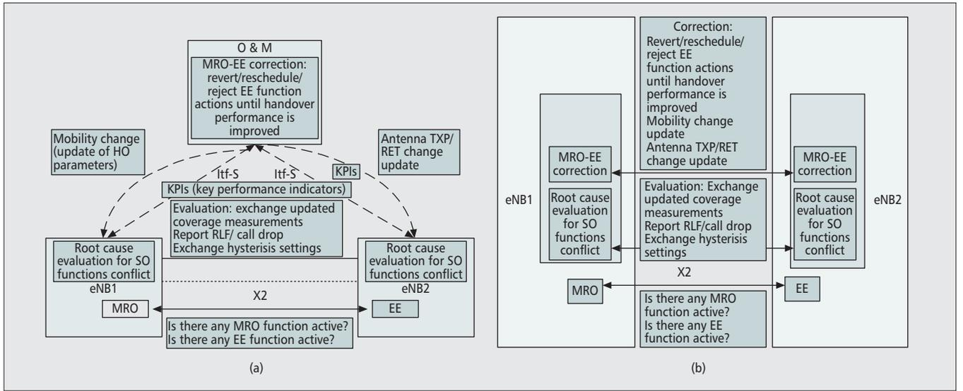
**Figure 3.** Hybrid self-coordination between MRO and EE functions: a) centralized architecture; b) distributed architecture.
