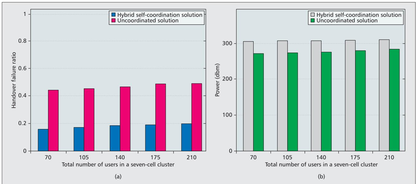
**Figure 5.** The performance evaluation of hybrid self-coordination between MRO and EE: a) the performance analysis of handover failure ratio; b) the performance evaluation of transmission power consumption.
