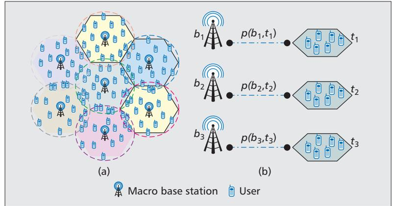
**Figure 4.** An illustration of a macrocellular network topology: a) an overview of a seven-cell macrocellular network; b) a graph-based representation of a macrocellular network.
