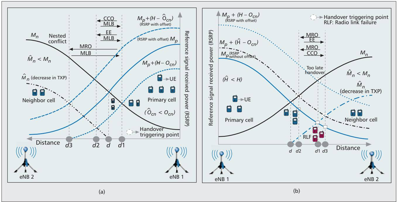
**Figure 1.** a) RSRP plot for illustration of conflict between MRO, EE, and CCO SON functions in multi-cell environments; b) RSRP plot for illustration of conflict between MLB, CCO, EE, and MRO SON functions in multi-cell environments.
